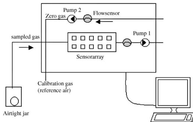
Fig. 1. Schematic diagram of the electronic-nose measurements and gas flow of PEN 2 during the experiments.
