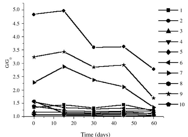
Fig. 4. Relative conductivity of each sensor vs. picking-date.
